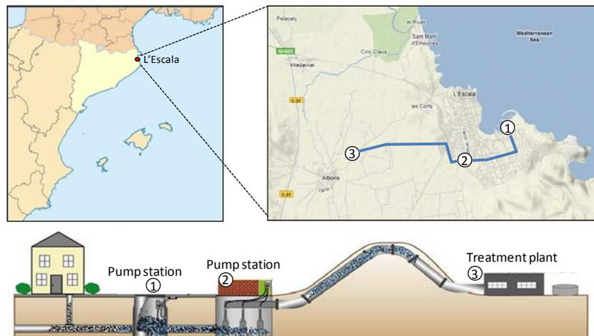
Figure 1. Location and scheme of l'Escala Urban Wastewater System with monitoring locations: ①&②: Pump stations; ③: Wastewater Treatment plant inlet.
