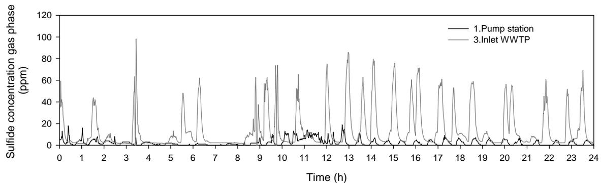
Figure 2. 24h profiles of H<sub>2</sub>S measured concentrations in the gas phase of points 1 and 3 of l'Escala UWS.
