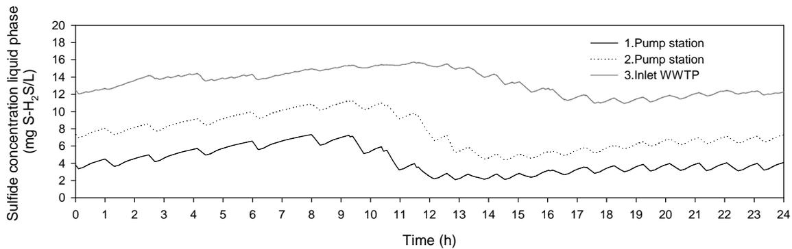
Figure 1. 24h profiles of Sulfide concentration predicted by the UQ sewer model in the different sections of the l'Escala UWS.
